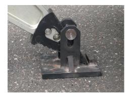
The TL-9 Stabilizer was designed by firefighters for firefighters! It allows you to perform a lift with your hydraulic spreader in a quick, efficient, and stable manner.
